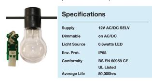
The Lumisphere® Carnival range of LEDs is a fully Dimmable AC/DC LED plug in light module which uses  $4\times5$ mm high brightness light emitting diodes mounted onto a conformal coated heavy duty PCB, with plug in connector ensuring a highly visible wide angle light source with low power consumption. The units are designed to operate at low temperature and drive currents to achieve maximum performance.
