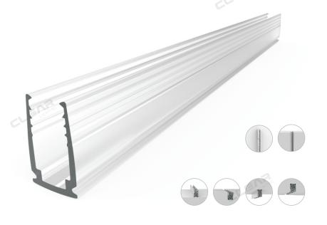
It uses thickened PC profile to 3mm thickness, specialized for underwater application up to 2m depth, and has excellent properties in rust, corrosion and fracture resistance.
