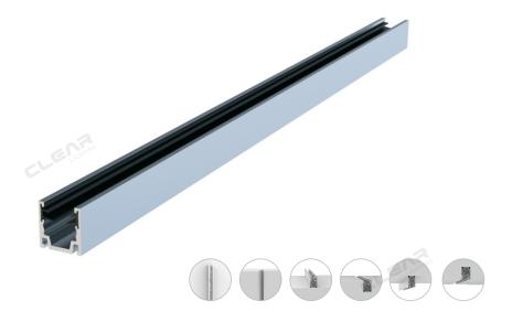
Specialized for the LED Flex Linear light, it was developed by combining the advantages of 6063 aluminum and elastic serrated tape. The inside elastic serrated tape as the grabbing force to keep continuous strong clamping force on the light body and protect the light from the damage caused by the large friction in the process of installation and dismantlement. It can stand max. 50 times of the light weight under -20~70°C and is easy to install and dismantle.
